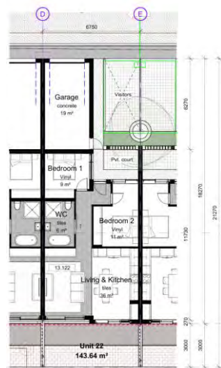
FIGURE 15: SINGLE STOREY UNIT LAYOUT (BPASS ARCHITECTS)
